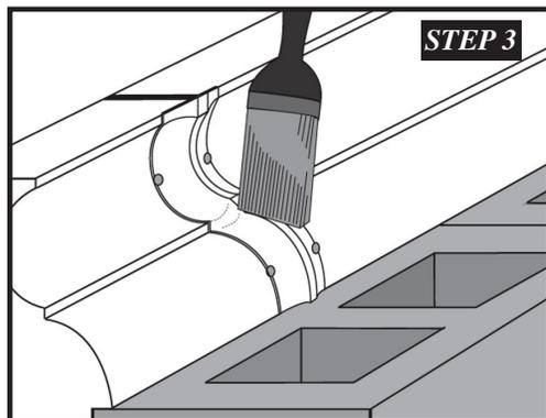
**Step 3.** Apply a coat of "Frontier Release Agent" to Chamfer Clip and allow to dry.
