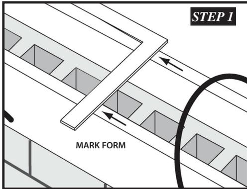
**Step 1.** Using a framing square, mark the location of the joints to be tooled.
