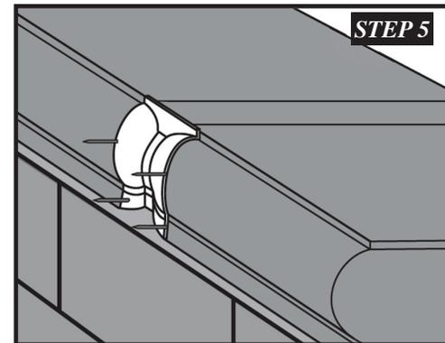
**Step 5.** Strip the Wall Cap form, exposing the Chamfer-Clip. Carefully remove the Chamfer Clip and wipe clean immediately for re-use.
