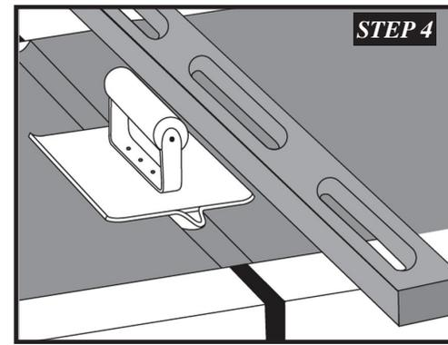
**Step 4.** Tool the joints at the appropriate time using the lay-out marks as a guide.
