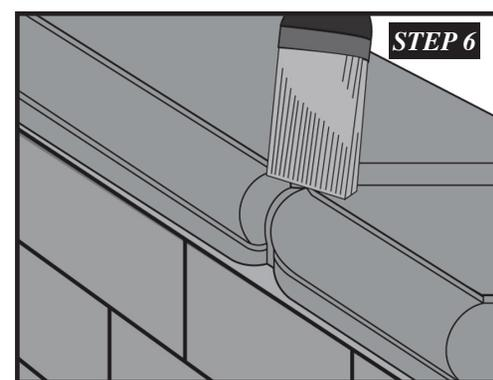
**Step 6.** Joints may be finished with a damp brush if desired.
