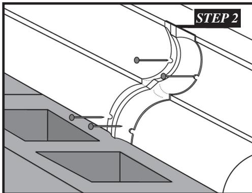
**Step 2.** Place the Chamfer Clip into the form and pin in place with the nails provided.
