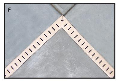
F. NOTE: Concrete must be edged to ensure future top cap removal. The fittings (90 degree, 45 degree, etc.) are supplied as "base only". During installation, the top caps (10 ft. long) run continuously over the fittings serving as a mounting device, leaving the fittings virtually invisible.
