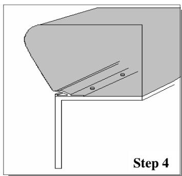
**Note:** Removing the forms one piece at a time will help keep the moisture in the concrete to allow adequate time to finish.
