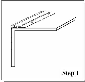
**Step 1.** Wipe the top and face of the pool wall with a clean cloth to remove any dirt or moisture. Place the track on the top of the pool wall as shown in the illustration. Line the bottom lip of the liner track flush with the face of the pool wall. Use the self-tapping screws provided to fasten the track down. It is important to have the track butted tightly together
