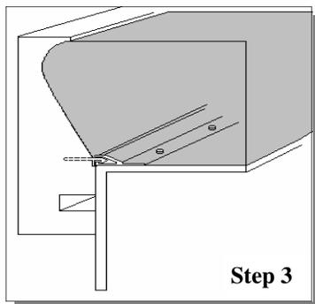
**Step 3.** While pouring tap the form to release air bubbles. This will help prevent honeycombing.
